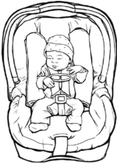
Figure 3: Car seat with a small cloth between crotch strap and infant, retainer clip positioned at the midpoint of the infant's chest, and blanket rolls on both sides of the infant.
